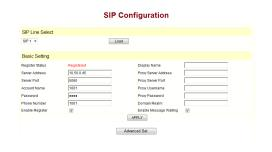
The Server Address of the IP/PBX, Extension Number/Account Name, Phone Number, Display Name, Enable Register, and Enable Message Waiting indicators are all programmed here.
