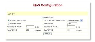
**VLAN Enable:** If enabled the traffic over the WAN port (and the bridged LAN port) will separate voice, signaling, and data transmission. This is an essential security feature in hospitality environments to separate voice on one Virtual LAN and guest data traffic on a second Virtual LAN.
