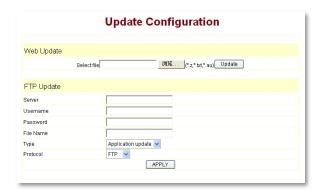
**Web Update:** Updates the application or configuration files of the phone. The telephone's firmware is in a .z format and the configuration files are in a .txt format.
