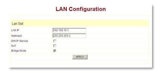
**LAN IP:** This is where you can set the IP address of the phone (at its LAN port). This is seldom used because in most environments Bridge Mode is enabled, causing the LAN port to act as a bridged extension of the WAN port.
