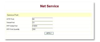
**Telnet Port:** Configures the Telnet transfer port; the default is 23.
