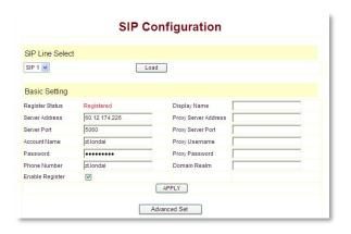
**Server Address:** This is the IP address or FQDN (Fully Qualified Domain Name) of the IP/PBX SIP Registration server.
