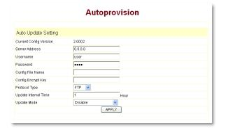
**Current Config Version:** The system displays the current version number.
