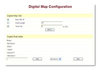
The digital map is a set of rules to determine when the user has finished dialing.
