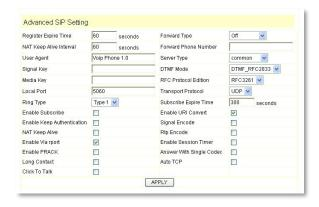
**Register Expire Time:** Registration expiration time. The default is 60 seconds. The I Series phone will automatically configure this expire
